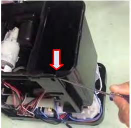
b.Push the water tank's fixed units
