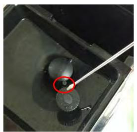
b.Remove the snap joints of the grinder supporter
