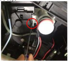
b. Push the brewing stopper gear case (as the direction of arrow)
