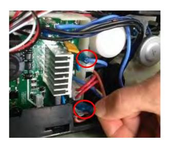
b.Remove the power switch E wire
