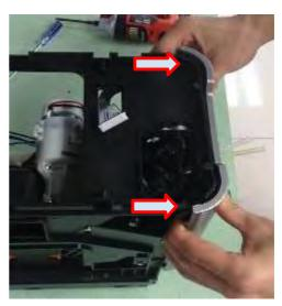
9. DISASSEMBLE WATER TANK'S FIXED COVER
