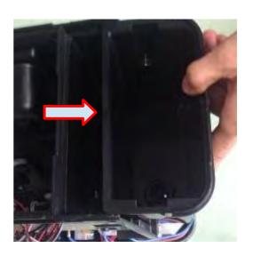
c.Pull the rubber hose and remove the fixed cover
