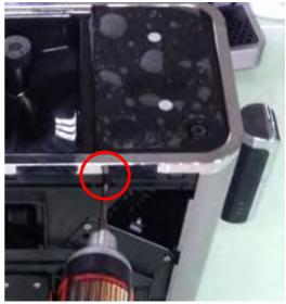
b. Remove the snap joints of the control panel
