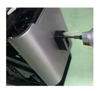
b.Remove the snap joints (of coffee lamp PCB)
