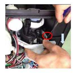
c. Take out the grinder after removing the two black lead wires
