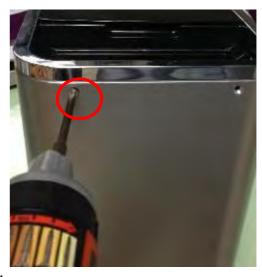
f.Remove the snap joints of the main body
